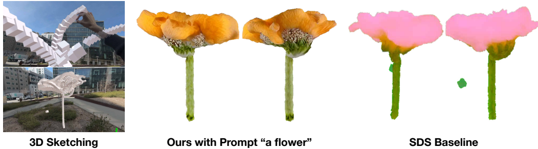
Figure 7: 3D sketch-to-real . We introduce a conditional generation task in 3D where a coarse human-drawn mesh is optimized into a high-quality mesh. While SDS and our gradient both adhere to the prompt and shape conditions, our method produces higher fidelity colors and texture.
